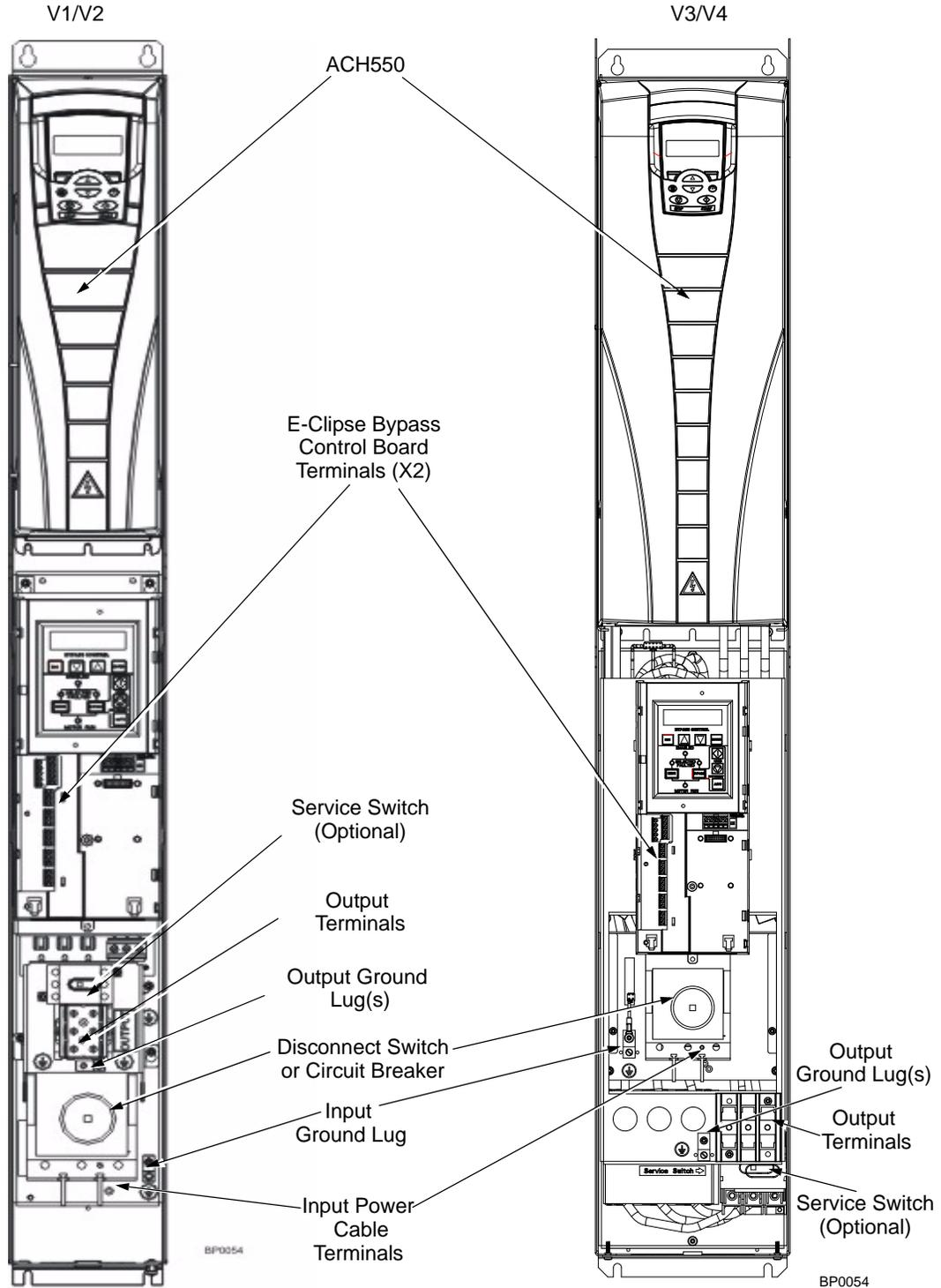
Connection Diagrams – Standard E-Clipse Bypass (Wall Mounted)
