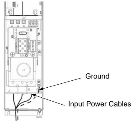
*Line Input Connections – Standard E-Clipse Bypass Configurations (Wall Mounted)*
