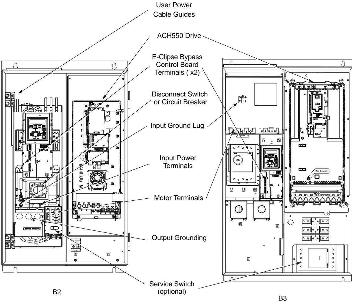
Connection Diagrams – Standard E-Clipse Bypass (R8, Floor Mounted)
