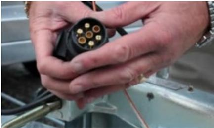
*Figure 17: pin lighting connector*
