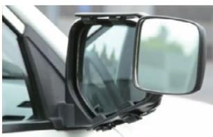
*Figure 12. Extension Mirrors also known as Towing Mirrors*
