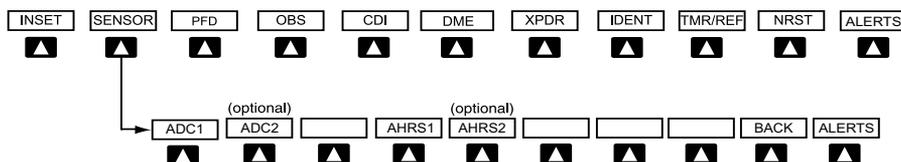
Press the **BACK** Softkey to return to the top level softkeys.
