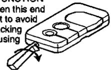
Replace cover as follows. *3-Function remote*: Insert the 3 tabs at the opposite end and snap shut.
