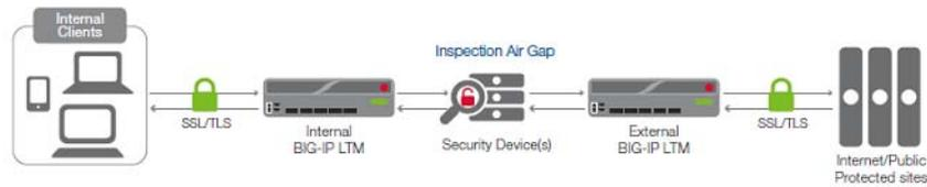
Figure 2: Air Gap Egress Inspection with SSL Intercept with multiple BIG-IPs
