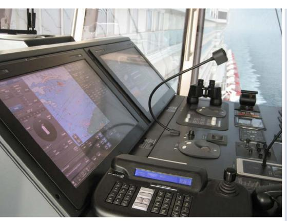
Designed with the help of ergonomics professionals, DP captains and ship controls experts, the Wärtsilä NACOS DP Platinum user interface represents a leap forward in intuitive ship controls. Full touch operation and screen layout engages the user while ensuring safer and more efficient operation. Only necessary and required information is presented, preventing confusion during critical operations.
