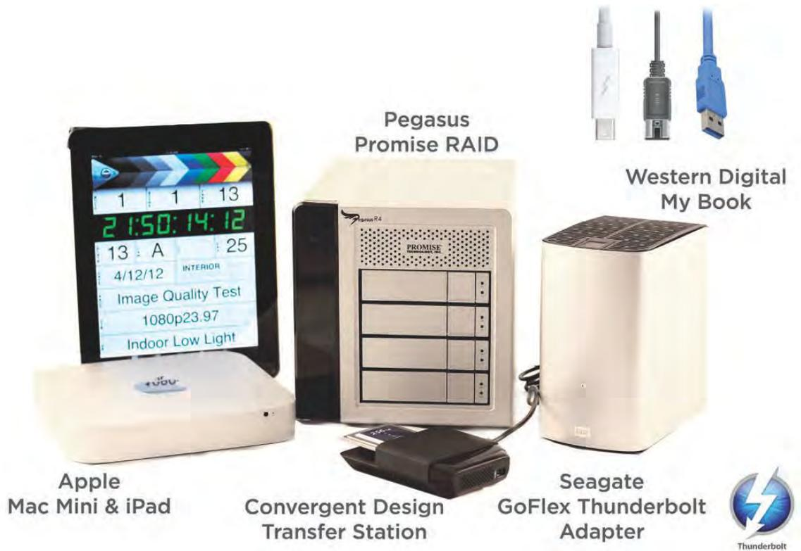
Example: Data can be transferred using a Mac Mini or Laptop via Thunderbolt, Firewire 800 or USB 3.0 to an external RAID (Pegasus Promise RAID shown) configured as a RAID 0. This can be used for live playback creating LOOK files or applying LUTs, as well as confidence monitoring of footage. We suggest having a secondary drive (Western Digital MyBook Studio shown, configured as a RAID 5 redundant), which can then make two simultaneous copies of the footage, for deliverables and archive.
