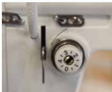
Tension Assembly with good spring (new Tension knob)
