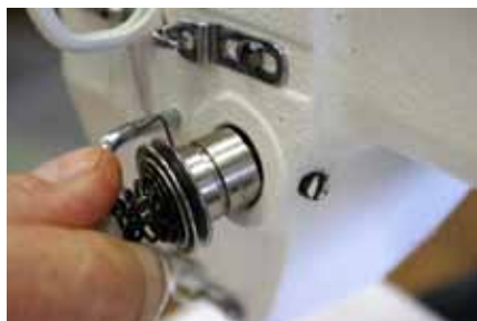
Remove assembly from machine Be careful of release pin
