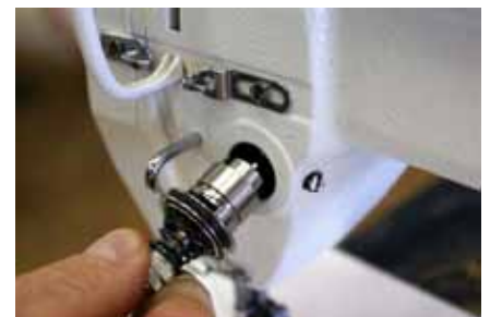
Place the assembly back into your machine Figure 90
