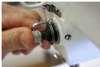
Press in and notice the tension disk opens Figure 92
