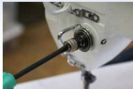
For fine adjustment of check spring insert screwdriver turn clockwise for more tension
