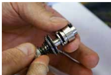
Remove tension assembly from barrel
