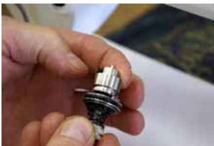
Give the tension assembly a twist until you feel resistance on the check spring Figure 88
