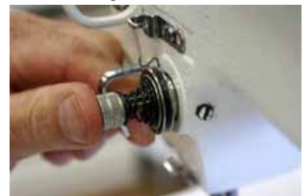
Release and the disk will close; this is the proper place for your tension assembly Figure 93
