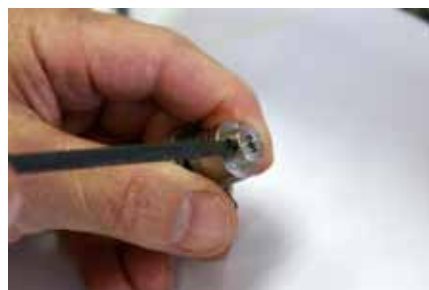
Loosen screw only DO NOT REMOVE
