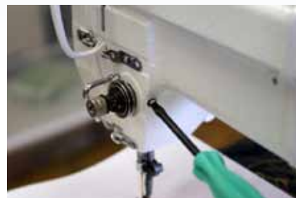
Screw on inside of machine loosen only. DO NOT REMOVE
