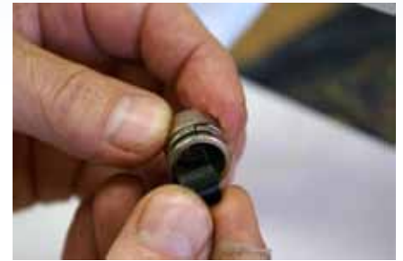
Twist while inserting the new spring Figure 84
