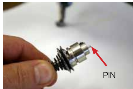
Tension assembly out of machine DO NOT LOOSE PIN
