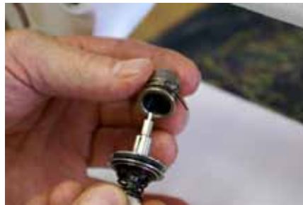
Insert the tension assembly back into the barrel. REMEMBER DO NOT LOOSE THE PIN Figure 86
