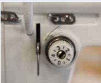
Tension assembly back in place with new check spring at 11:00
