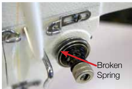
Tension Assembly with Broken Spring. (old tension knob)
