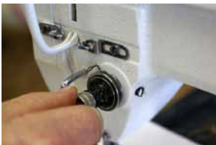
Once in insure that your check spring is at 11:00 Figure 91
