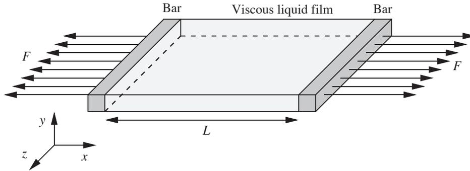
Fig. P6.1 Stretching of liquid film between two bars.
