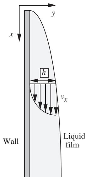
Fig. P6.5 Liquid draining from a vertical wall.
