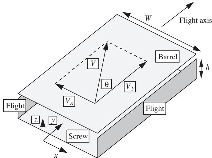
Fig. E6.4.2 Diagonal motion of barrel relative to flights.
