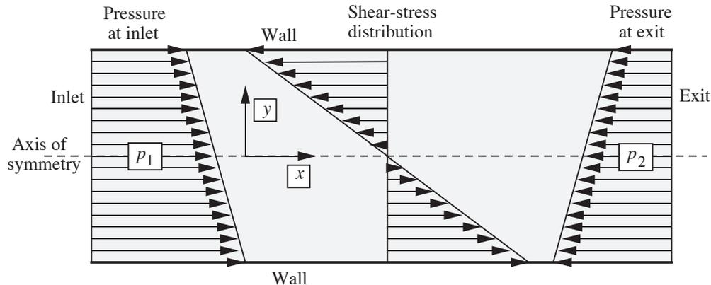
Fig. E6.1.3 Pressure and shear-stress distributions.
