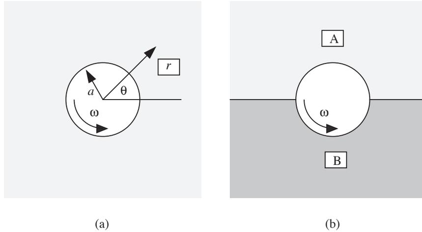
Fig. P6.19 Rotating cylinder in (a) a single liquid, and (b) two immiscible liquids.
