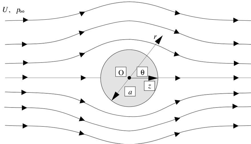
Fig. P6.12 Viscous flow past a sphere.
