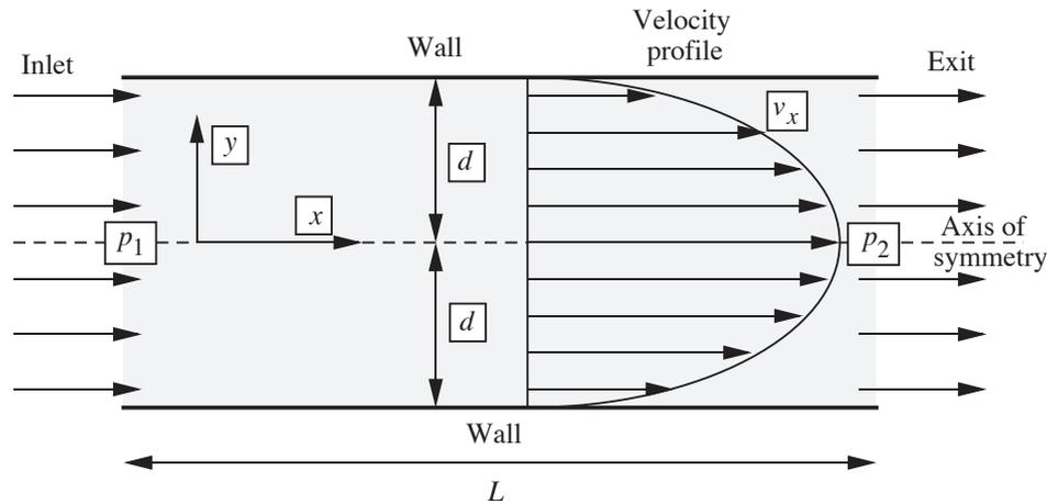
Fig. E6.1.2 Geometry for flow through a rectangular duct.
