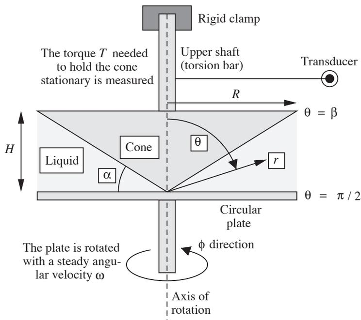
Fig. E6.7 Geometry for a Weissenberg rheogoniometer.
