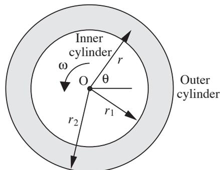
Fig. P6.13 Section of a Couette viscometer.
