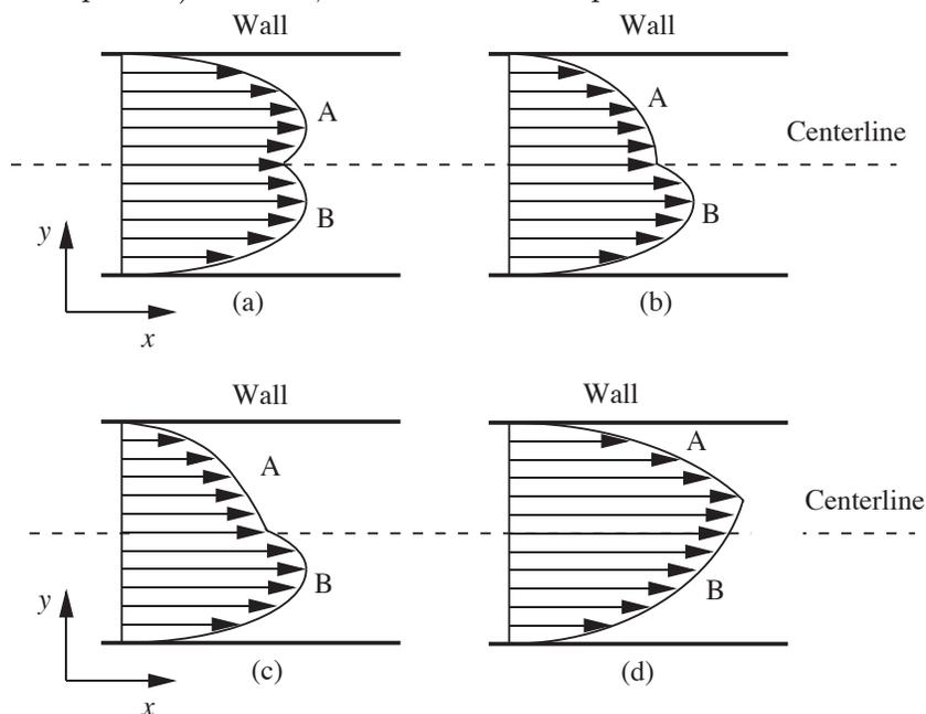
Fig. P6.11 Proposed velocity profiles for immiscible liquids.
