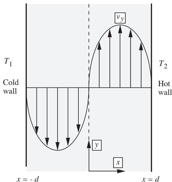
Fig. P6.8 Natural convection between vertical walls.
