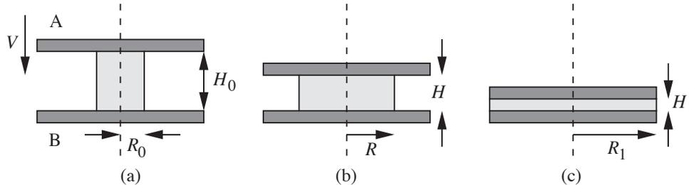
Fig. P6.4 Compression molding between two disks.
