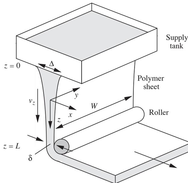
Fig. P6.6 “Spinning” a polymer sheet.
