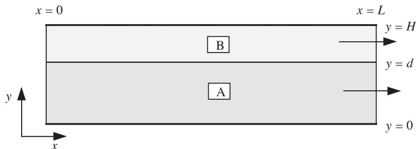
Fig. P6.20 Two-phase flow between parallel plates.
