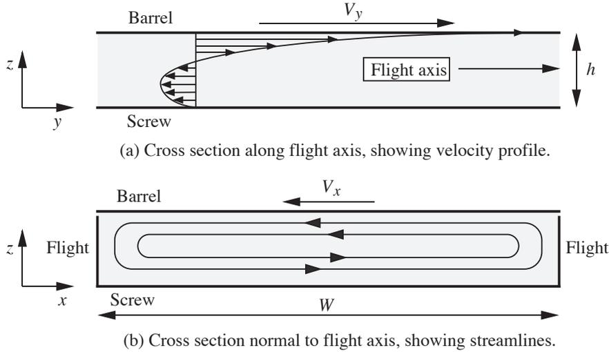
Fig. E6.4.3 Fluid motion (a) along and (b) normal to the flight axis, as seen by an observer on the screw.
