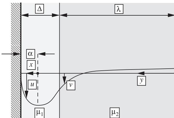
Fig. P6.24 Flow of two immiscible liquids in a pipe.
