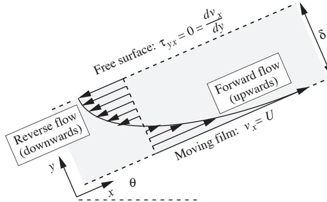
Fig. E6.3.2 Velocity profile in thin liquid layer on moving photographic film for the case of zero net liquid flow rate.
