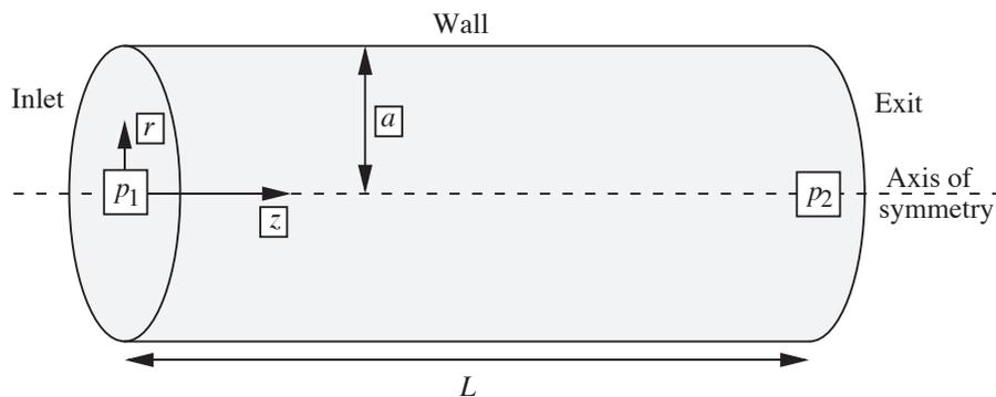
Fig. P6.7 Flow of a liquid in a horizontal pipe.
