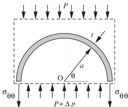
Fig. P6.25 Cross section of half of a cylindrical bubble.
