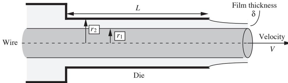
Fig. P6.2 Coating of wire drawn through a die.
