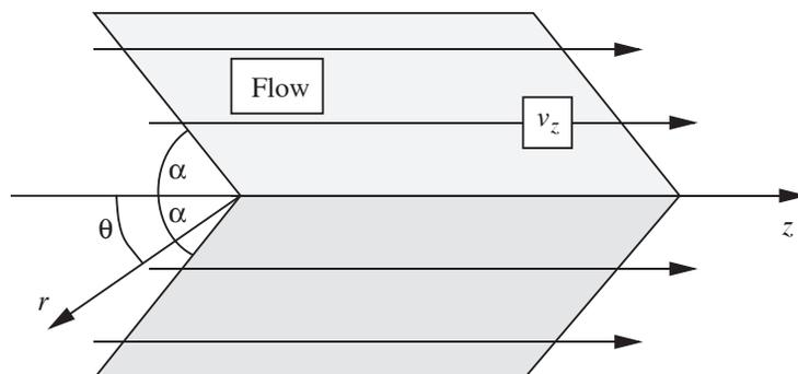
Fig. P6.23 Flow between inclined planes.
