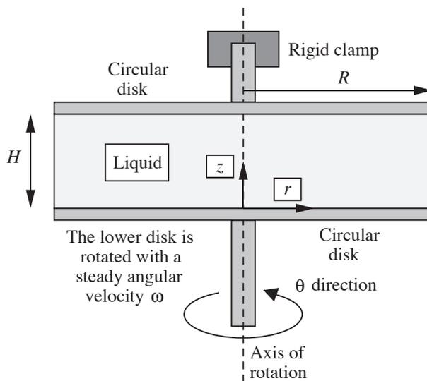
Fig. P6.16 Cross section of parallel-disk rheometer.
