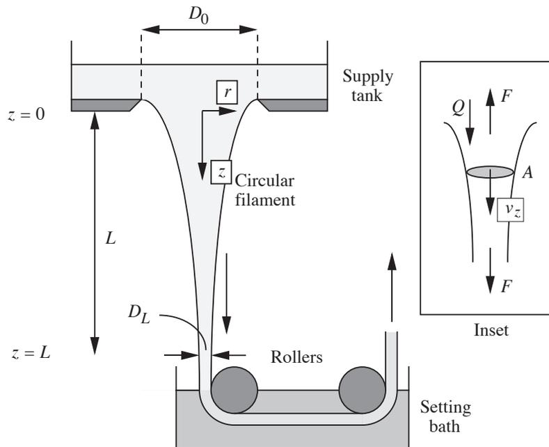
Fig. E6.6 “Spinning” a polymer filament, whose diameter in relation to its length is exaggerated in the diagram.
