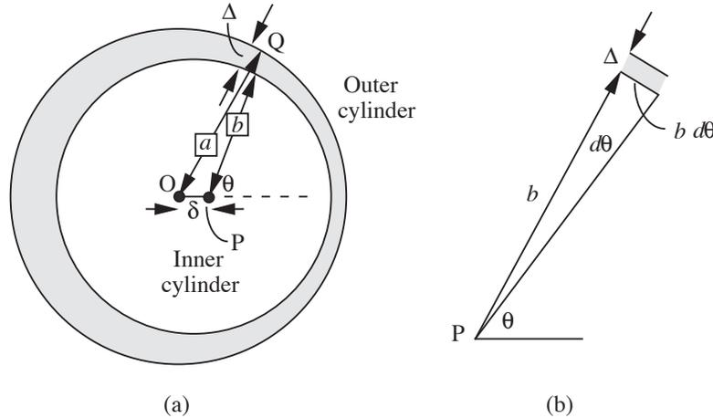
Fig. P6.3 Off-center cylinder inside a die (gap width exaggerated): (a) complete cross section; (b) effect of incrementing  $\theta$ .
