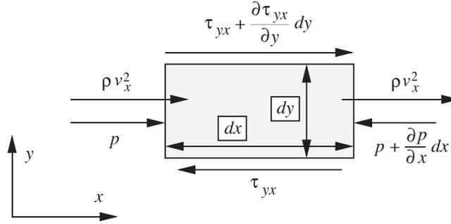
Fig. E6.2 Momentum balance on a fluid element.
