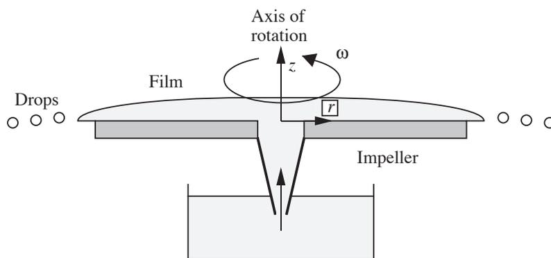
Fig. P6.21 Rotating-impeller humidifier.
