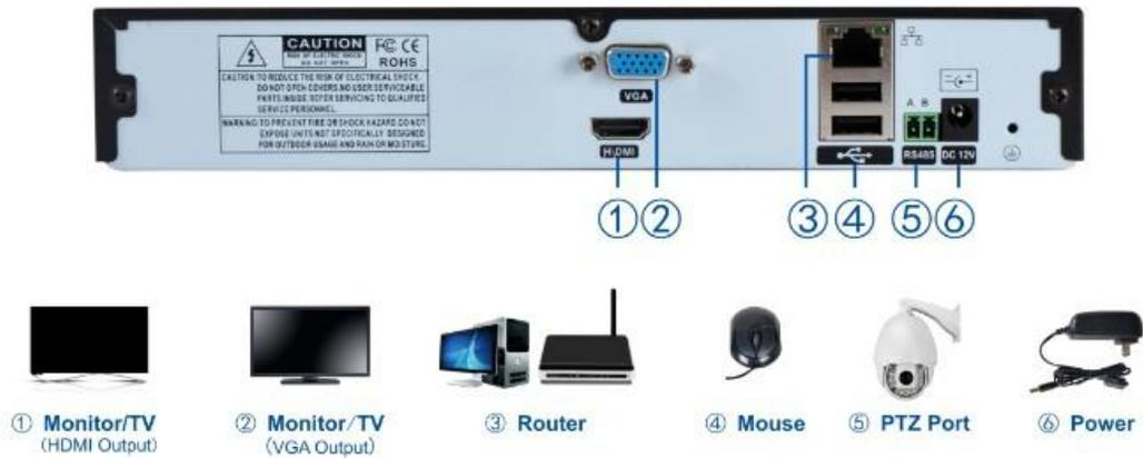
NVR Connections: Diagram 2
