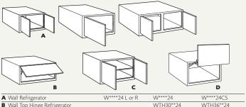
WTH30\*\*24 WTH36\*\*24 B Wall Top Hinge Refrigerator W/24\*\*24 L or R W\*\*\*\*24CS C Wall Refrigerator w/Shelf W/\*\*\*\*74 W\*\*\*\*24 D Wall Refrigerator Vertical Lift
