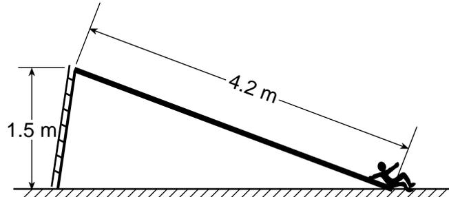
71–72 Calculate the speed of the child at the instant she reaches the bottom of the slide. [Show all work, including the equation and substitution with units.] [2]
