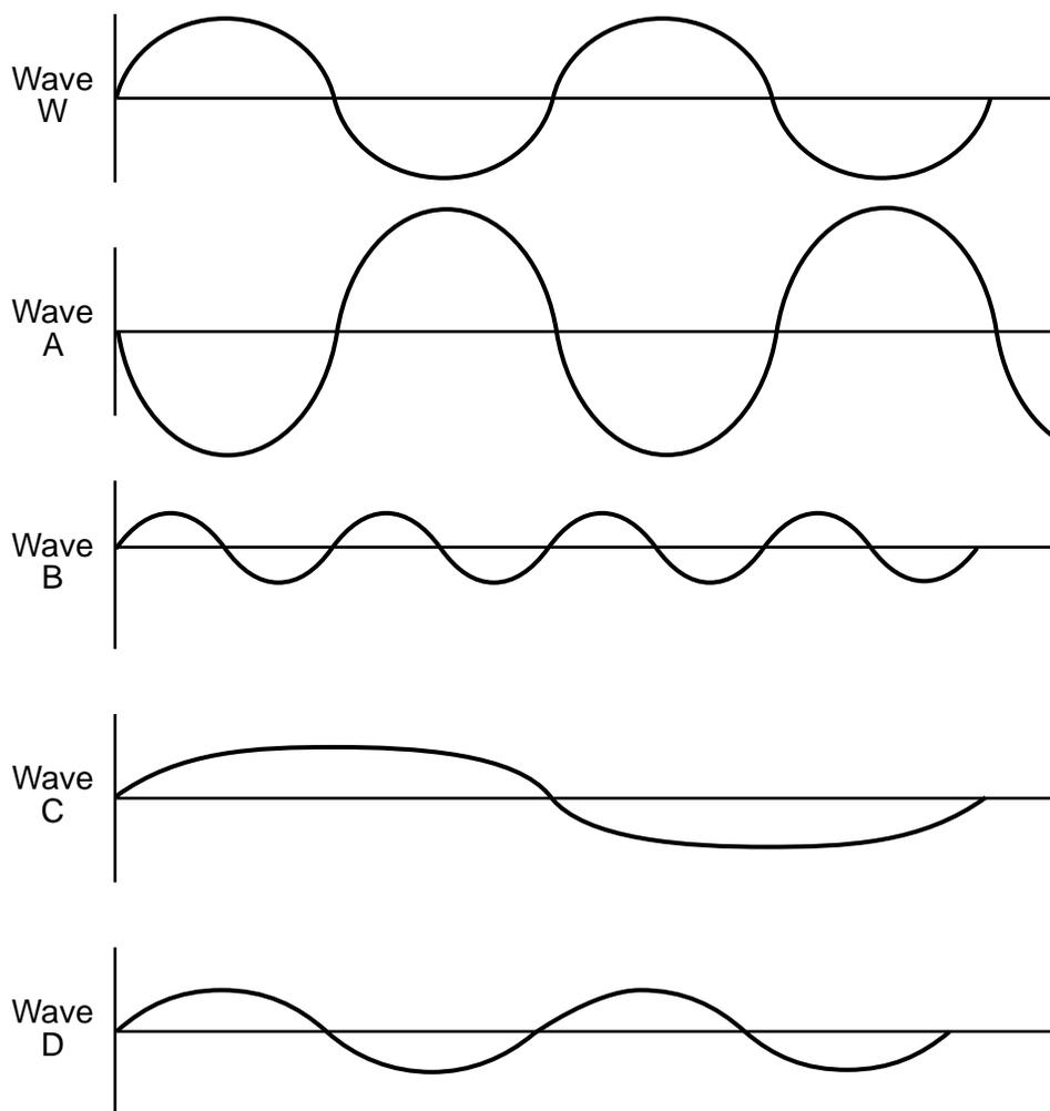
46 Which wave has a period that is twice that of wave *W*?
