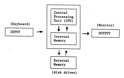
The Central Processing Unit (CPU) or microprocessor is the heart of the computer. The power and speed of a microcomputer depends greatly on the type of processor. Different types of processors are (increasing speed and therefore price) 8088, 80286, 80386 and 80486.
