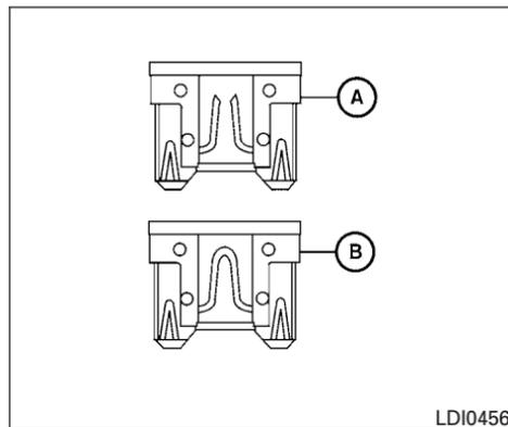
5. If the fuse is open (A), replace it with an equivalent good fuse (B).
