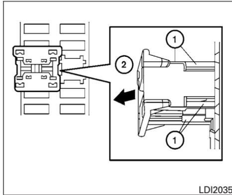
How to replace the extended storage switch:
